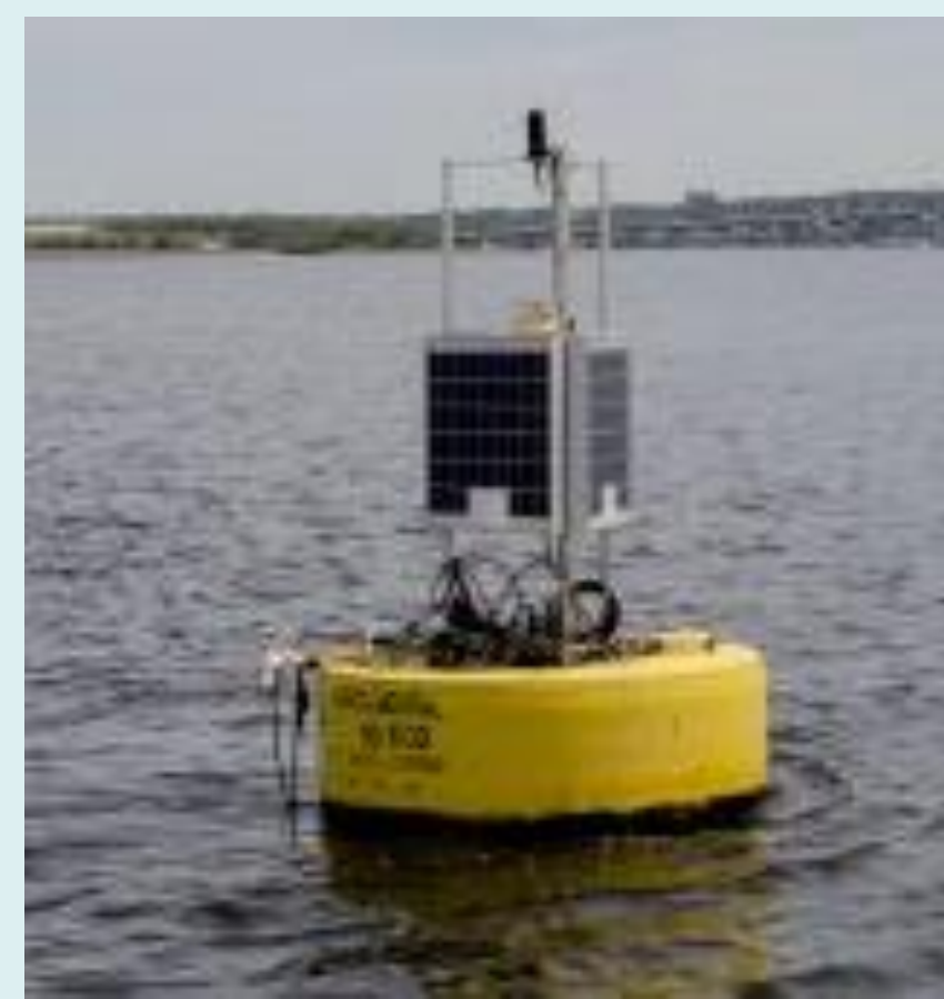
PICTURE. NBFSMN buoy with continuous, remote water quality monitoring equipment attached.
