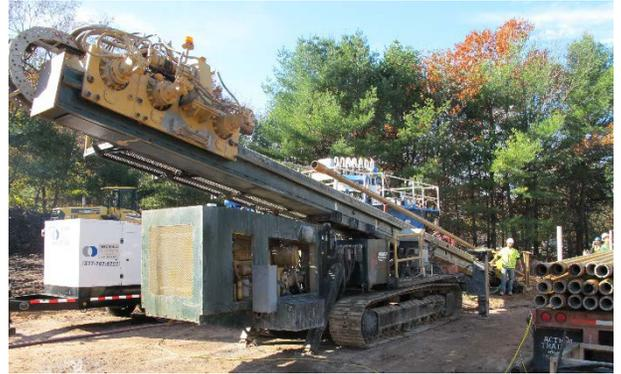
Directional drilling is the specific drilling practice of controlling the direction and angle of a wellbore to a specific location. This technique can be used to achieve a number of different goals including drilling multiple wells from one location, to reach inaccessible surface locations and multiple target zones, or to place pipeline beneath major roadways and even cross waterways with minimal disruption.
